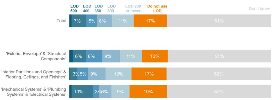
If LODs are used, we see that the installation parts (mechanical, plumbing, and electrical) are more detailed – meaning LOD 400 or 500 – than other building parts
